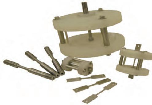
High temperature-high pressure vessels is comparable for use with AI stress ring, slow strain stress corrosion and corrosion fatigue testing machine.
